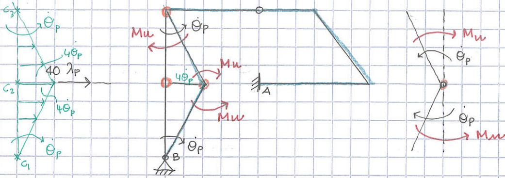
$$P = \lambda_p 40 \dot{\theta}_p u - M_u (\dot{\theta}_p + \dot{\theta}_p + \dot{\theta}_p) = 0 \quad \forall \dot{\theta}_p \Rightarrow \lambda_p = \frac{3 M_u}{160} = \frac{3 \cdot 500}{160} = \frac{75}{8} \sim 9,37 > \lambda_s \quad (\checkmark)$$
