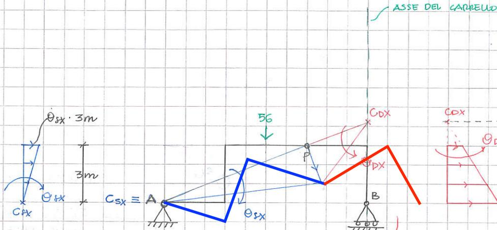
$$\begin{aligned} \delta v(P)_{sx} &= \theta_{sx} \cdot 7 \text{ m} \\ \delta v(P)_{dx} &= \theta_{dx} \cdot 3 \text{ m} \end{aligned}$$
