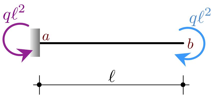
$$T(s) = 0 \quad \rightarrow \quad M(s) = \text{const.}$$
