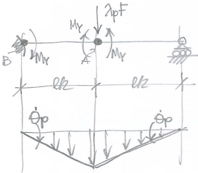
$$2M_y \dot{\lambda}_p \text{ in A} \\ 1M_y \dot{\lambda}_p \text{ in B}$$
