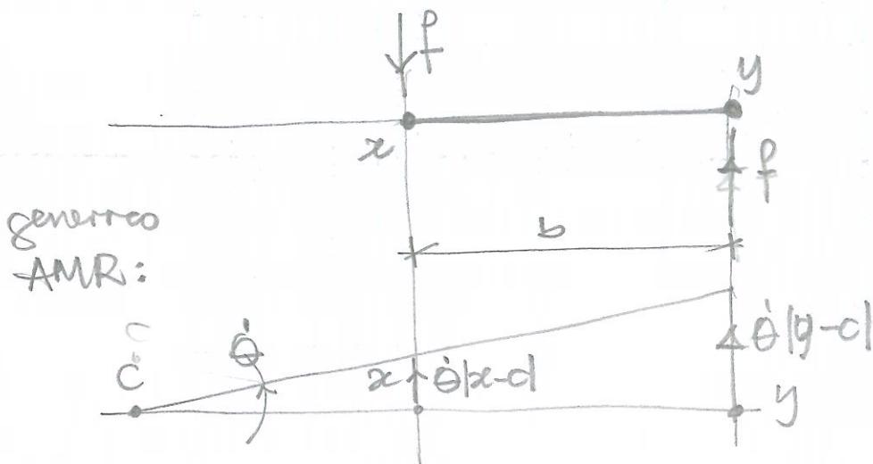
$$\begin{aligned} P &= -f \dot{\theta} |x - c| + f \dot{\theta} |y - c| \\ &= f \underbrace{(|y - c| - |x - c|)}_b \dot{\theta} = f b \dot{\theta} \end{aligned}$$
